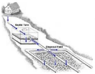
Common in rural areas without centralized sewer systems, OSS are underground wastewater treatment structures that use a combination of nature and time-tested technology to treat wastewater from household plumbing produced by bathrooms, kitchen drains, and laundry.
